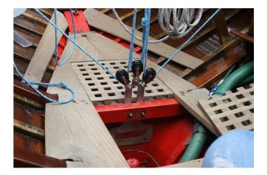
Three single blocks are attached to a custom fitting (cut by Fibre Fusion's water jet) bolted to the aft-most oak floor. The floor carries one of the long vertical bolts securing the external lead keel (864kg) so is a very safe anchorage for the mainsheet load.
